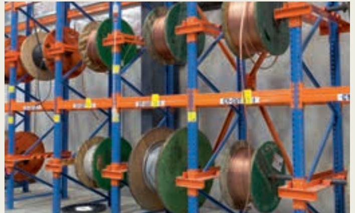
CABLE REEL RACKING
